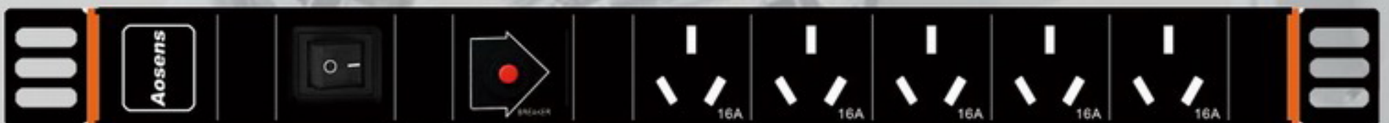
型号 Model: AS-1U-J5KG 尺寸 Size: 430*44.4*44.4mm 额定电流 16A, 5位16A国标孔, 总控开关(带指示灯), 过载保护 16-Amp rated current/5 16-amp Chinese outlets/ One 16-amp general control switch (indicator)/ One 10-16amp overload protector
