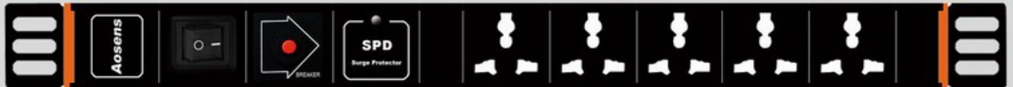
型号 Model: AS-1U-M5KGF 尺寸 Size: 430*44.4*44.4mm 额定电流10- 16A, 5位10A万用孔, 总控开关(带指示灯), 过载保护, SPD防雷(浪涌)保护功能(带指示) 10-16Amp rated current/5 10-amp international outlets/ One 16-amp general control switch (indicator)/ One 10-16amp overload protector/ One SPD LED
