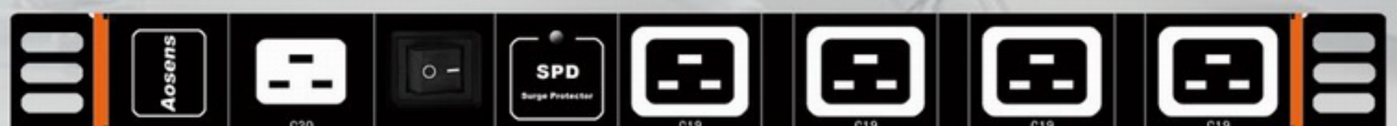
型号 Model: AS-1UB-D4KF/B 尺寸 Size: 430*44.4*66.6mm 额定电流 16A, 4位IEC60320-C19 16A输出孔, 总控开关(带指示灯), SPD防雷(浪涌)保护功能(带指示), 16A IEC60320-C20 输入 16-Amp rated current/4 16-amp IEC60320-C19 outlets/ One 16-amp general control switch (indicator)/ One SPD LED/1 16-amp IEC60320-C20 inlets
